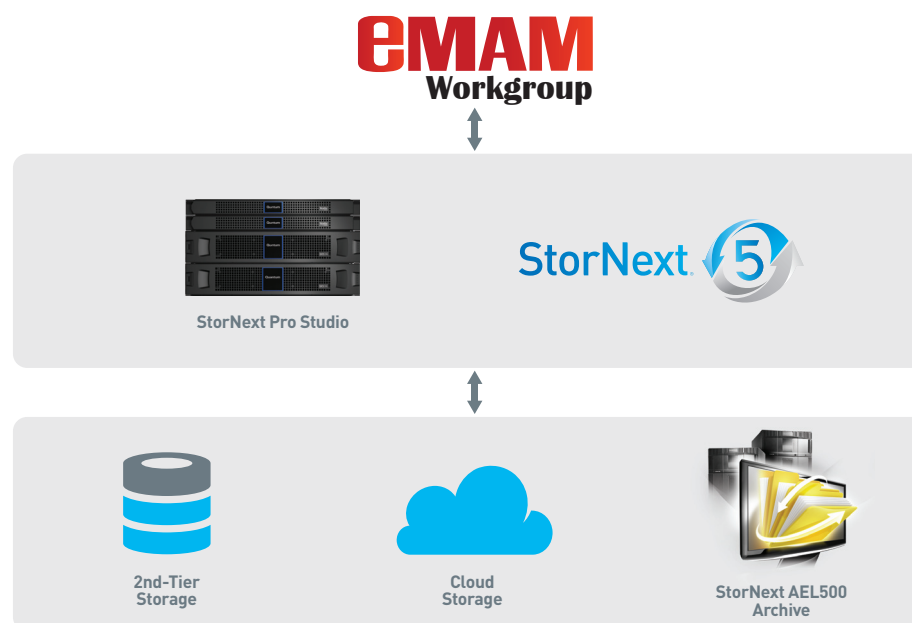
Figure 1. The StorNext Storage Manager manages and optimizes movement of content from 1st-Tier storage to less-costly 2nd-Tier storage to Cloud and/or Archive according to administrator-defined policies. eMAM Workgroup provides a powerful, yet easy-to-use and flexible interface for review, approval, archive/restore, and collaborative workflows.
